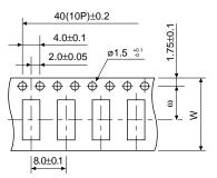
SSP-T5/T6 (Conforms with IEC60286-3)
